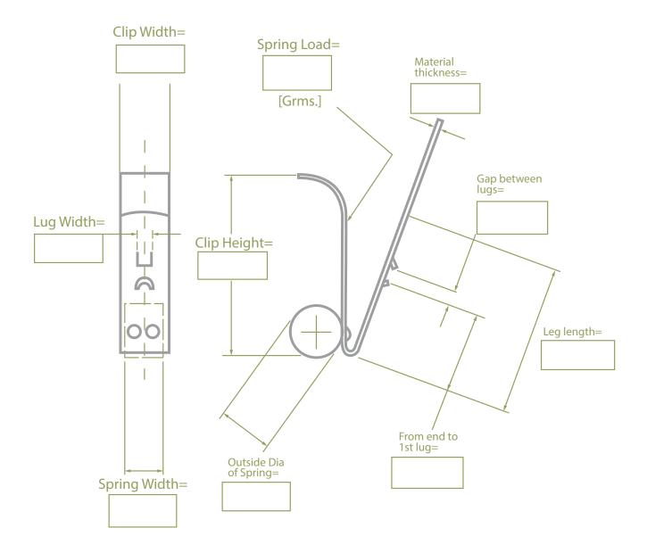
For the purpose of quotation (prior to sending any damaged / broken spring clips through to us), please advise the
